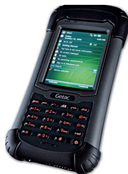
11-nji surat. SDR 31/33 kysymly elektrton meýdan kompýuteri
