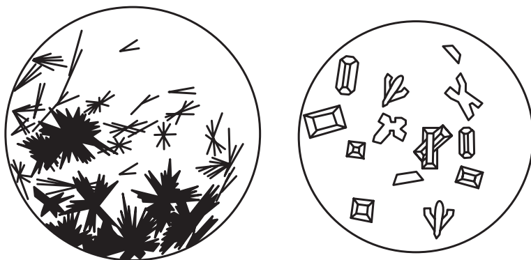
3.1-nji surat. Duzlaryň erginlerden kristallaşmagyndan alnan \text{CaSO}_4 \cdot 2\text{H}_2\text{O} we \text{Mg}(\text{NH}_4)\text{PO}_4 \cdot 6\text{H}_2\text{O} kristallary (mikroskop astynda)
